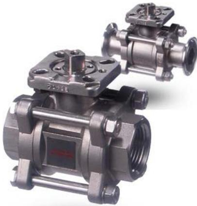
The 36 is a full port, 316 stainless steel, 3 piece ball valve. It is available with threaded ends (36N), socket weld ends (36S), or quick clamp ends with cavity filler seats (36CPF). It can be equipped with a manual handle or with pneumatic or electric actuators.
